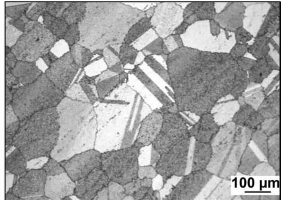
Fig. 3. Optical micrograph of the solutionized Nimonic 115.
