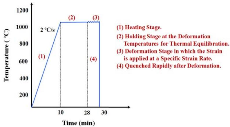
Fig. 5. The heating and deformation schedule.
