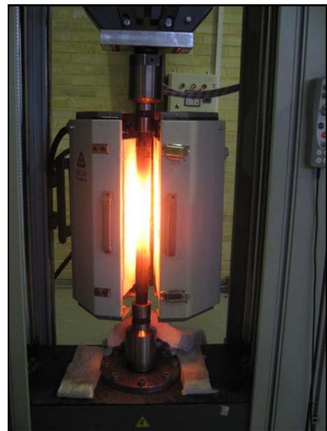
Fig. 4. Hot compression test machine.
