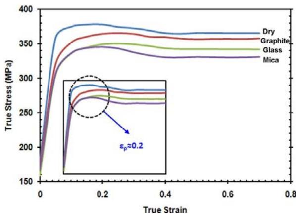
Fig. 6. True stress-strain curves Nimonic 115 at 1100 °C.
