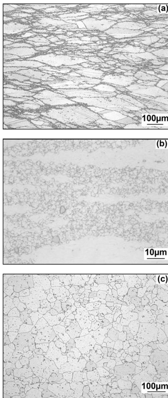
Fig. 8. Optical micrographs of Nimonic deformed with strain rate of  $1 \text{ s}^{-1}$  at different temperatures of (a)  $1100^\circ\text{C}$ , (b) necklace structure at  $1100^\circ\text{C}$ , and at (c)  $1175^\circ\text{C}$ .
