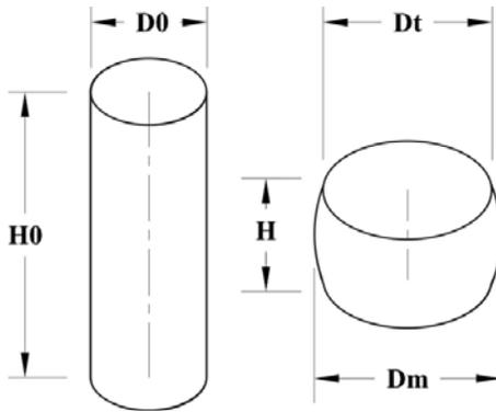
Fig. 2. Cylindrical compression test geometry.
