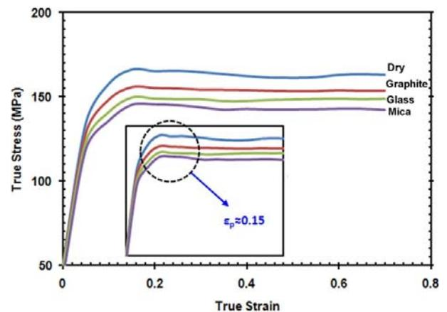
Fig. 7. True stress-strain curves Nimonic 115 at 1175 °C.
