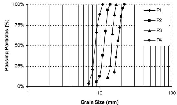
FIG. 3: Grain size distribution of porous media.
