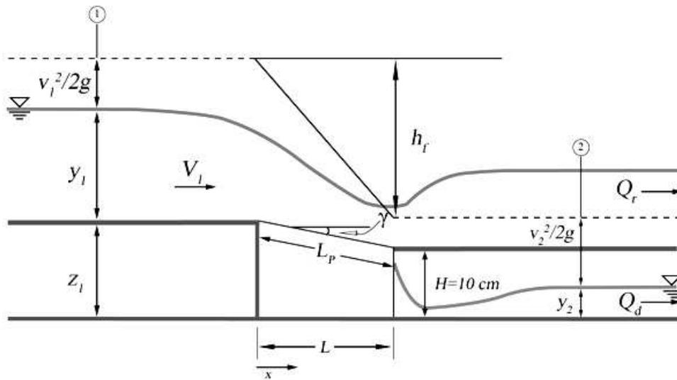
FIG. 9: Hydraulic characteristics of the flow in the bottom intake with porous media.
