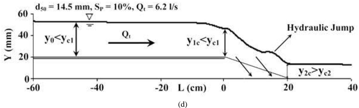
FIG. 5: Different types of water surface profiles on bottom intake with porous media.
