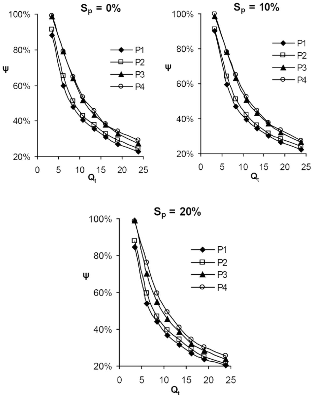
FIG. 4: Effect of grain size distribution on  $\psi$  variations in different surface slopes.
