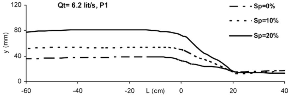
FIG. 8: Water surface profiles in different slopes of intake ( $Q_t = 6.2$  L/s and grain type P1).
