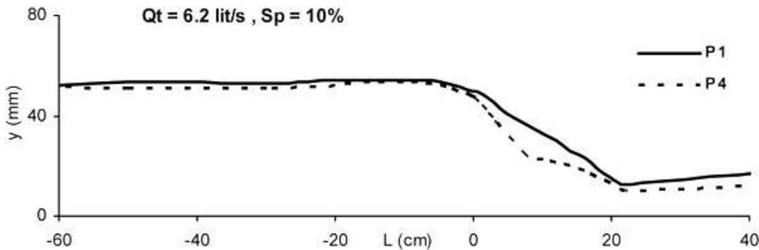
FIG. 7: Water surface profiles for grain types P1 and P4 ( $Q_t = 6.2 \text{ L/s}$ ,  $S_p = 10\%$ ).
