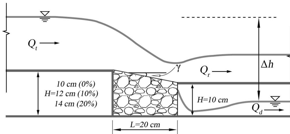
**FIG. 1:** Sketch of water intake frame as trench of porous media with different heights.
