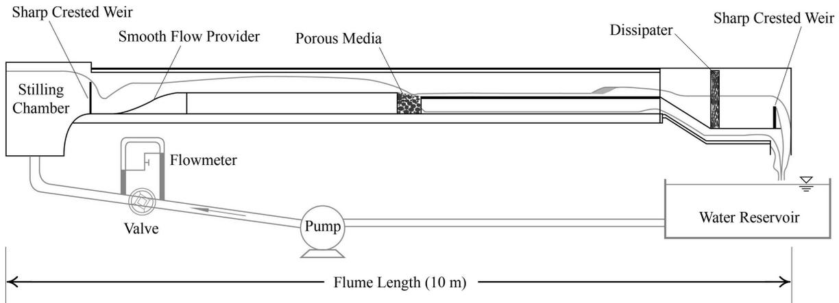
FIG. 2: Longitudinal section of the experimental setup.
