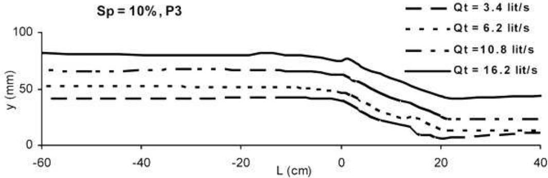
FIG. 6: Water surface profiles in different discharges (grain type P3,  $S_p = 10\%$ ).
