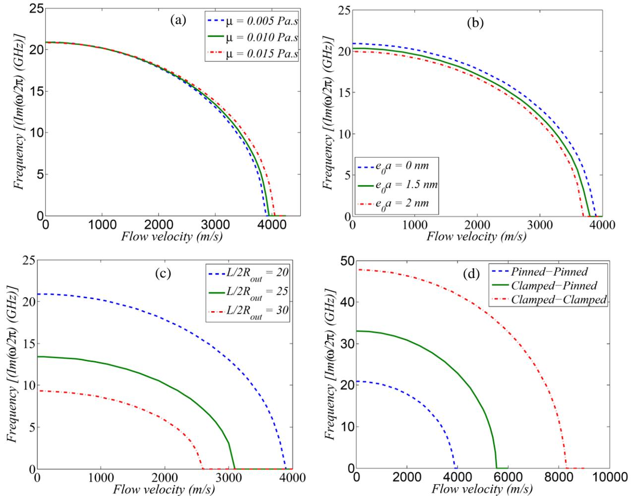
**Figure 1.** Fundamental frequencies of a pinned-pinned CNT as a function of flow velocity for different, (a) viscous parameters, (b) nonlocal parameters, (c) aspect ratios and (d) boundary conditions.
