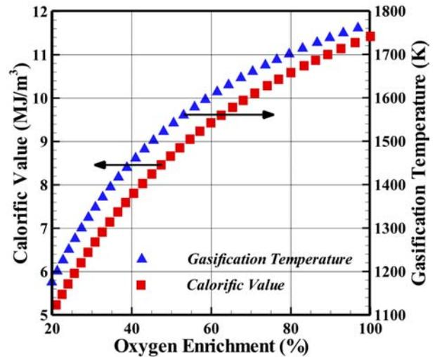
Fig. 2. Effect of oxygen enrichment on gasification temperature and calorific value of the syngas
