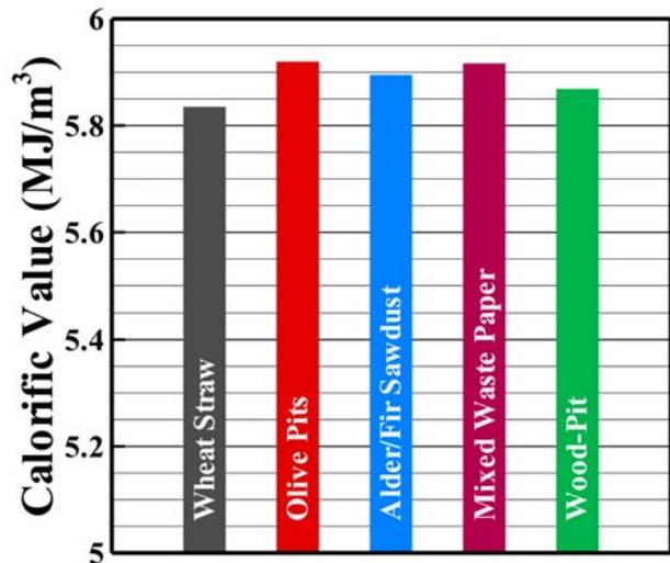
Fig. 1. Comparison between calorific values obtained via gasification of five different biomass materials
