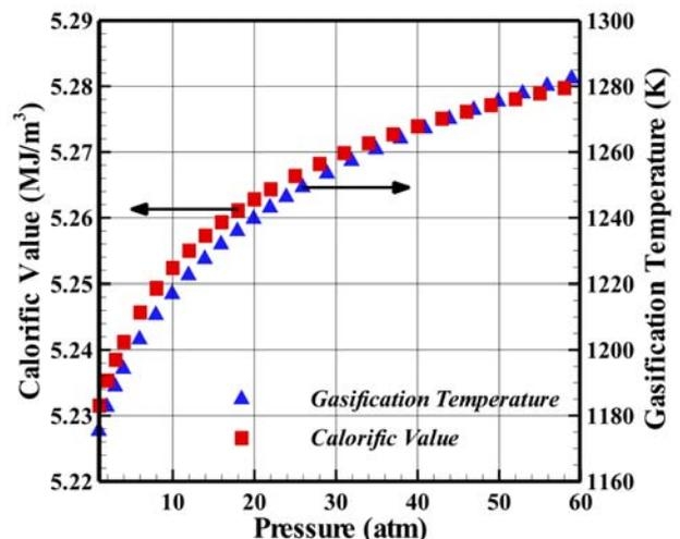
Fig. 4. Influence of pressure on gasification temperature and calorific value of the syngas.
