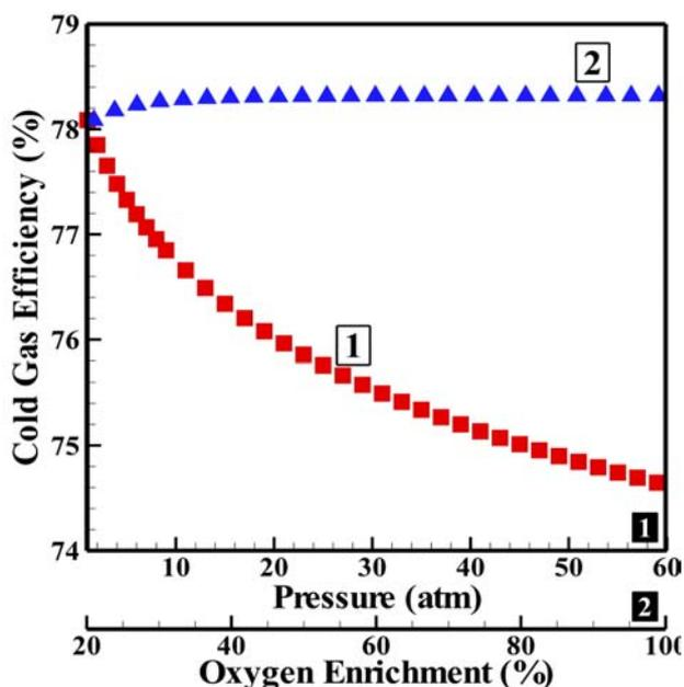
Fig. 6. Effect of oxygen enrichment and pressure on cold gas efficiency
