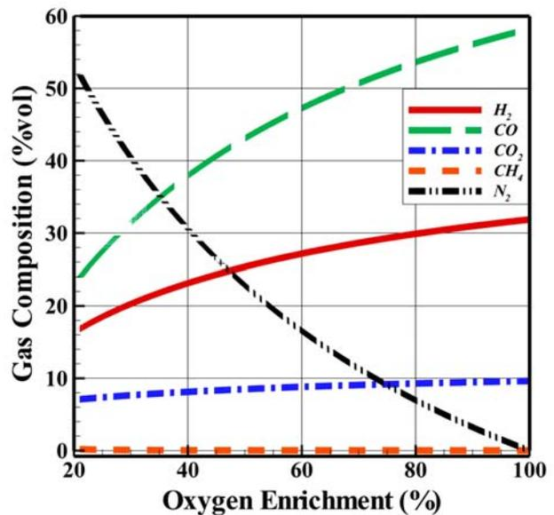
Fig. 3. Effect of oxygen enrichment on gas composition
