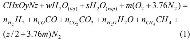
where  $x$ ,  $y$ , and  $z$  are numbers of atoms of hydrogen, oxygen, and nitrogen per one atom of carbon in the feedstock; respectively, and  $w$ ,  $m$ , and  $s$  are molar quantity of moisture, air/oxygen, and steam, respectively. All inputs on the left-hand side of Eq. 1 are defined at 25°C. On the right-hand side,  $n_i$  is the number of moles of species  $i$ , which is an unknown. Molar quantity of water per one kmol of biomass can be written as [11]:
