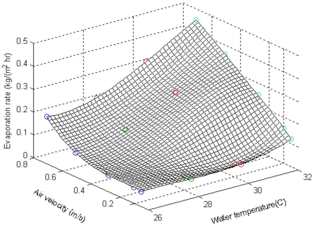
**Figure 2** Effect water temperature and air velocity on free water surface evaporation rate
