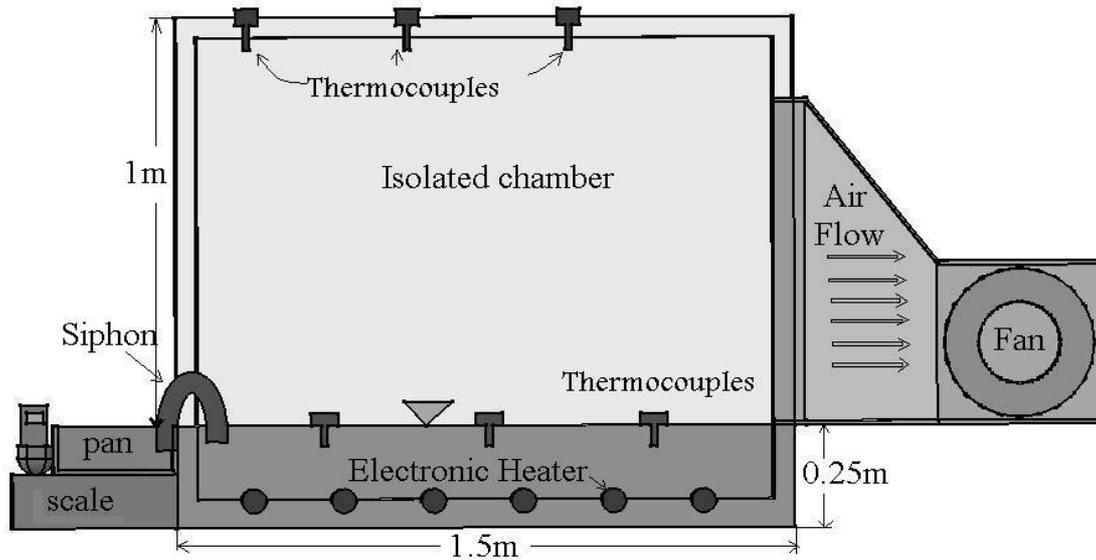
**Figure 1** Experimental test chamber and its essential features
