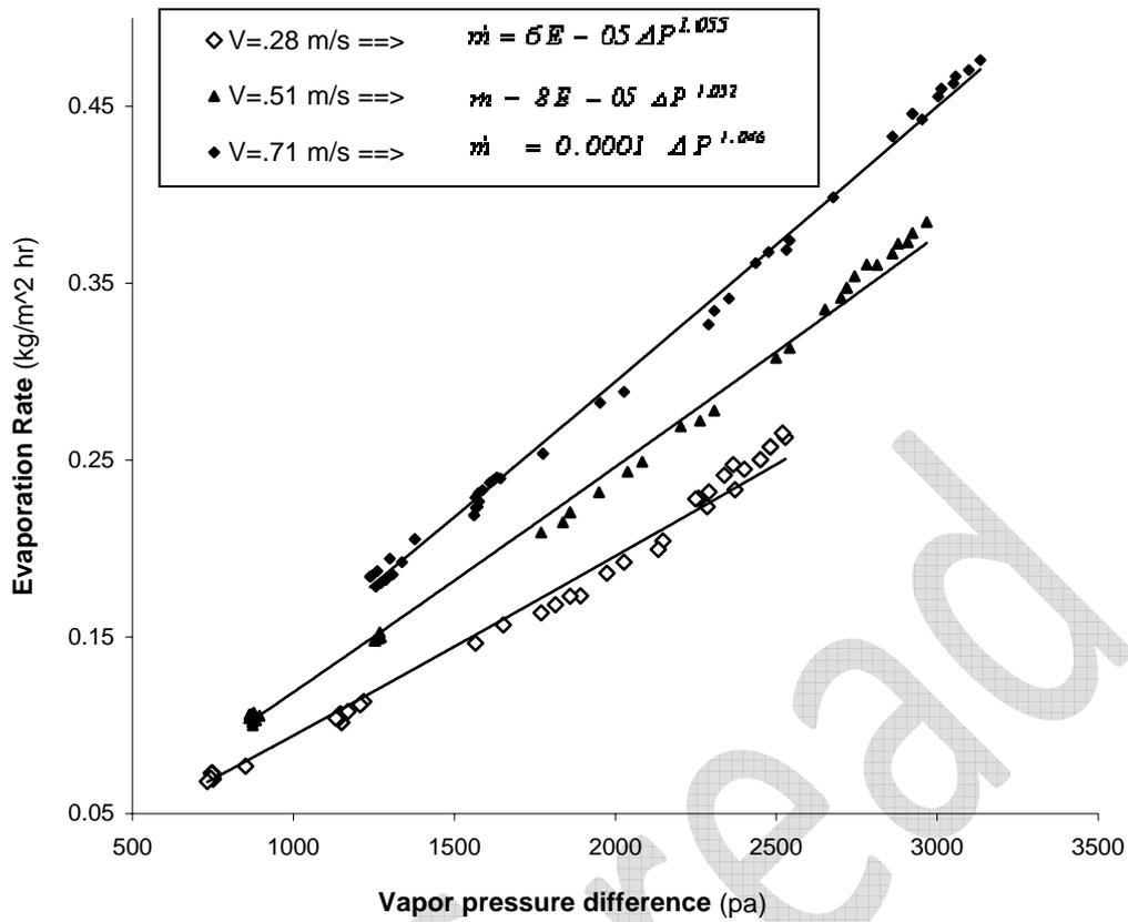
Figure 4 Effects of vapor pressure difference and air velocity on water evaporation rate
