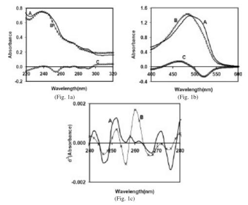
Fig. 1. Absorbance spectra of thorin and Be-thorin in the range of (a) 220-320 nm, (b) 400-600 nm and (c) third derivative in the range of 240-280 nm, at pH 10.5. Curve A is reagent blank (thorin  $4.8 \times 10^{-3}$  %) (reference, water), curve B is mixture of 0.2 µg mL<sup>-1</sup> of Be<sup>2+</sup> and  $4.8 \times 10^{-3}$ % of thorin (reference, water), curve C is Be-thorin; their concentrations are as in curves B (reference, reagent blank)
