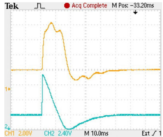
Fig. 16. Experimental results for the phase jump of 40^\circ : Ch1 denotes the estimated frequency (4 Hz/div), Ch2 denotes the phase error (15°/div).
