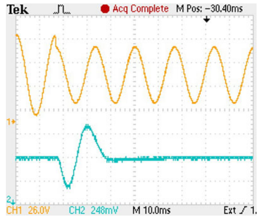
Fig. 20. Experimental results for voltage sag of 30%: Ch1 denotes the input voltage (26 V/div), Ch2 denotes the phase error (1.5° /div).
