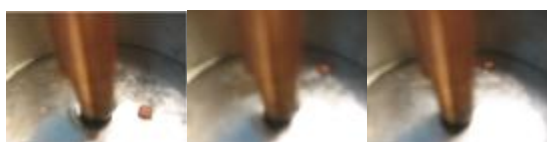
Fig. 8. Picture frames of the marker motion on the LM level due to the tangential Lorentz force
