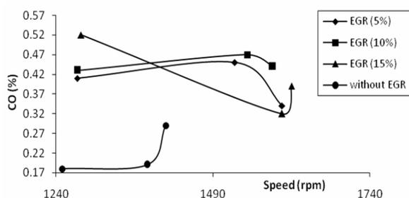
Figure 2. Effect of engine speed variations on CO emission of dual fuel HCCI-DI engine
