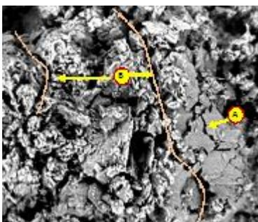
Figure 3: The fracture of grains (A) and vertical crack (B) due to 10 blows on Aq Emam hill
