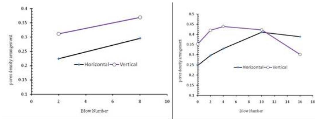
Figure 12: The changes of pores density arrangement due to dynamic blows on Loess samples of Aq Emam (right) and Hutan (Left)
