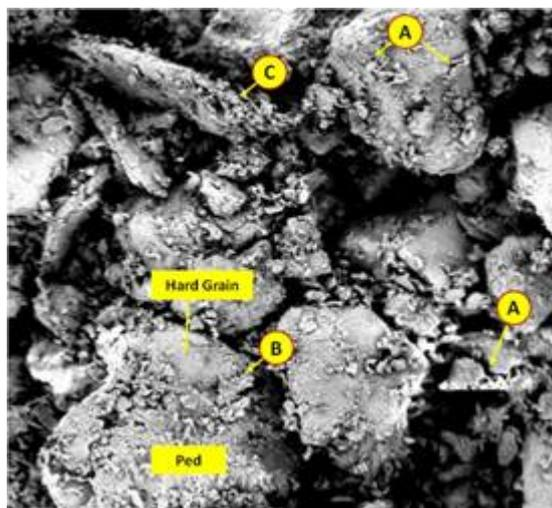
Figure 7: Breaking the grains (A), submerge of resistant grains in aggregate (B) and disintegration of mica particles (C) due to 8 blows on Hutan sample.
