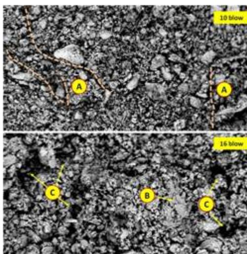
Figure 4: Microstructure changes due to 10 blows (above figure) and 16 blows (bottom figure) on Aq Emam samples. Explanation: Cracks (A), grains fracture (B) and crack (C) But in Hutan samples, the reduction of the size of grains is considerable and this is due to the break behavior in the soil. In this sample, the aggregate is broken and is changed into fine grains (Fig. 5).
