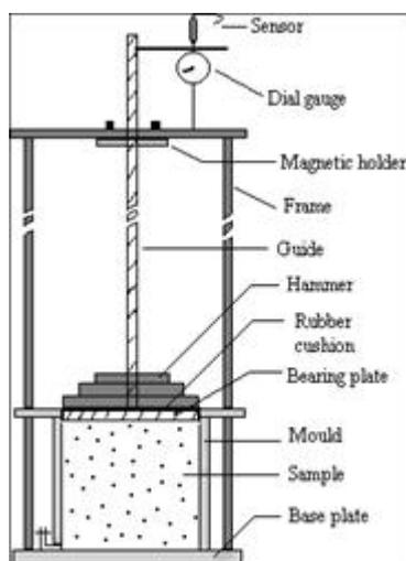
Figure 1: Schematic of dynamic compaction apparatus (Hu et al. 2001).
