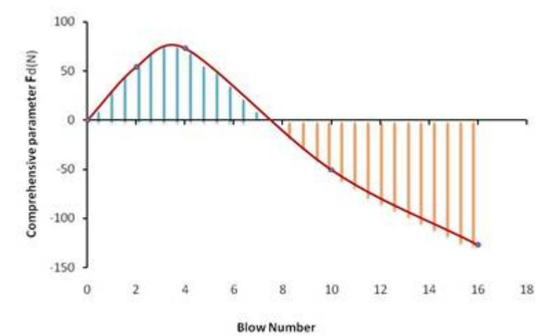
Figure 16: The effect of blow dynamic compact on comprehensive microstructure parameter of Loess
