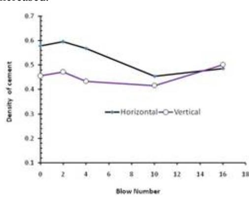
Figure 14: The changes of cement density arrangement due to dynamic blows on Loess samples of Aq
