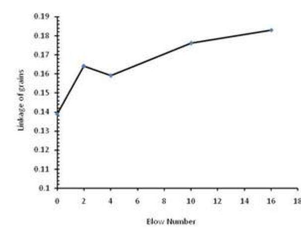
Figure 13: The changes of the connectivity between the grains due to dynamic blows on Loess samples. It is due to the increase of the break of connectivity between the grains and the closeness of the grains. The density of cement distribution between the grains in Aq Emam hill is increased in the initial blows but it is reduced to 10 blows and it reaches the constant value. As cement distribution density in horizontal and vertical directions approach in high blows.
