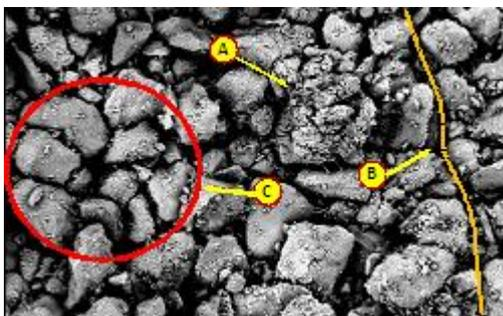
Figure 5: Aggregates fracture (A), vertical crack (B) and new arrangement of grains (C) due to 2 blows on Hutan sample
