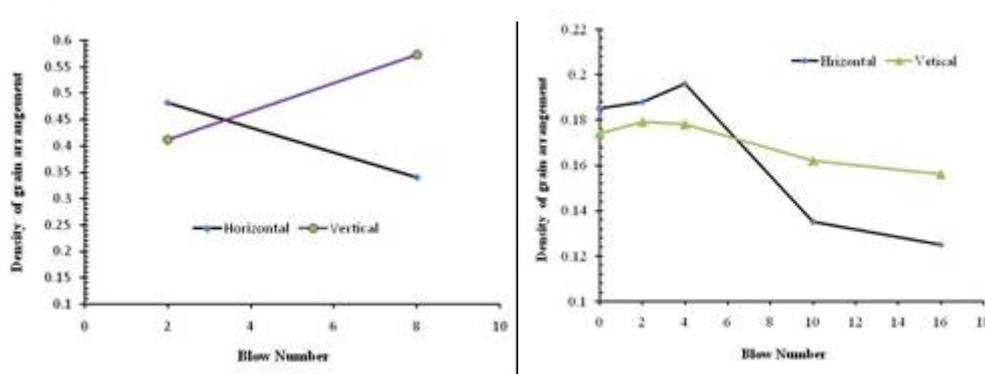
Figure 9: The dynamic compaction effect on density arrangement of AqEmam hill Loess grains (right) and Hutun (left)
