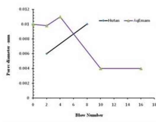
Figure 11: The changes of pores diameter due to dynamic blows on loess samples of Aq Emam and Hutan. In Hutan samples, by increase of blows, the diameter of the pores are increased. This is due to the fact that in Aq Emam hill samples, the soil behavior was plastic and by blows, the pores are small but in Hutan samples, the soil is brittle and bigger porous space is created.
