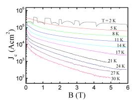
FIG. 1. The  $J_c$ -field dependence obtained from the M-H loops at different temperatures measured on a Ba<sub>0.72</sub>K<sub>0.28</sub>Fe<sub>2</sub>As<sub>2</sub> single crystal.
