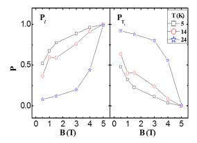
FIG. 4. Magnetic field dependences of the  $\delta l$  and the  $\delta T_{\rm c}$  pinning contributions in Ba<sub>0.72</sub>K<sub>0.28</sub>Fe<sub>2</sub>As<sub>2</sub> single crystal at different temperatures.
