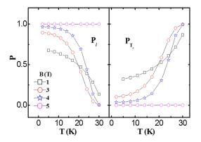
FIG. 3.  $\delta l$  and  $\delta T_c$  pinning contributions as functions of temperature in Ba<sub>0.72</sub>K<sub>0.28</sub>Fe<sub>2</sub>As<sub>2</sub> single crystal at different magnetic fields.
