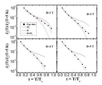
FIG. 2. Temperature dependence of the normalised measured current density  $J_c$  at magnetic fields of 1, 3, 4, and 5 T. The solid lines are the theoretical curves obtained based on the model of the  $\delta l$  (blue curves) pinning mechanism, the model of the the  $\delta T_c$  (black curves) pinning mechanism, and the coexistence of both (red curves) pinning mechanisms.
