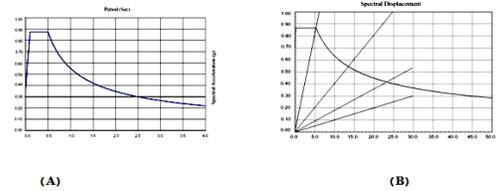
Figure 4-A: spectral acceleration -period curve, B-spectral displacement - spectral acceleration curve
