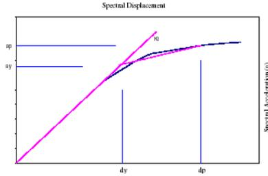
Figure 5- bilinear capacity spectrum
