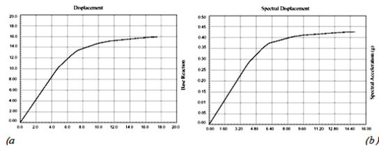
Figure 3-A: capacity curve, B: capacity spectrum
