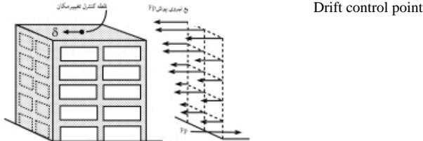
Figure 1- an example of loading on the building for the static nonlinear analysis [10]
