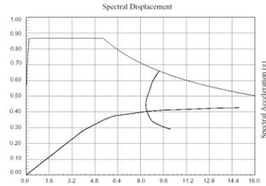
Figure 6- finding the performance point by the precise method
