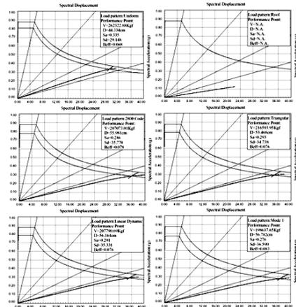
Figure 9- finding the performance point of 25-story structure with the precise method for the different load patterns
