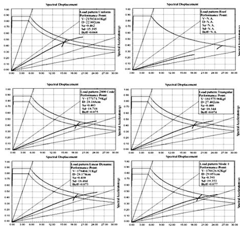
Figure 8- finding the performance point of 15-story structure with the precise method for the different load patterns
