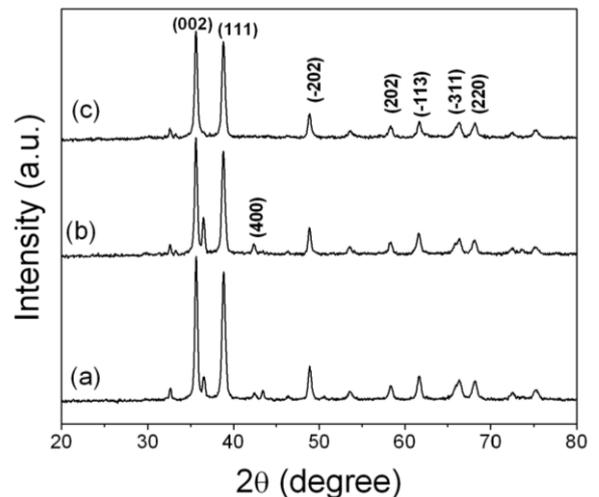
Fig 1. XRD Pattern of CuO:Fe nanoparticles with a)5% b)10% and c)15% of Fe content.
