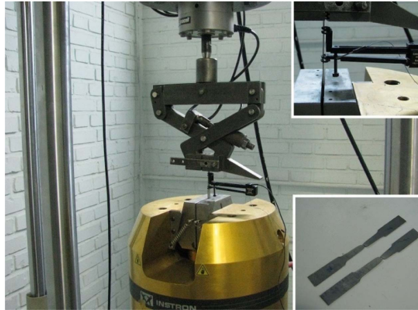
Fig. 1 Simple tension test according to ASTM E8 standard
