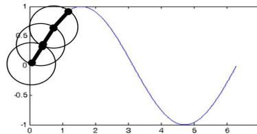
Fig. 12. Fitting snake robot links to body curve
