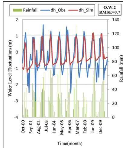
Figure 5. Comparison of observed and simulated water level fluctuation with WTF model for OW2.
