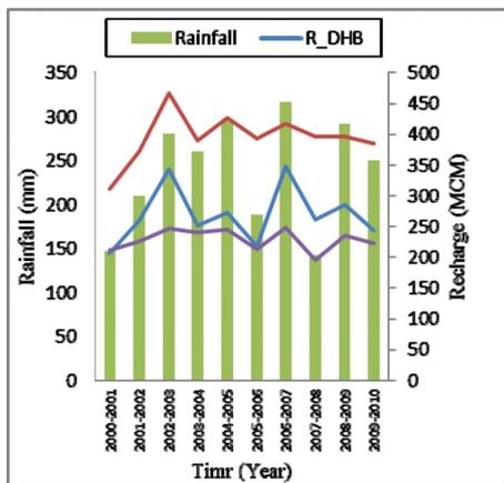
Figure 4. Comparison between groundwater recharge estimated through HB, DHB and WTF methods.
