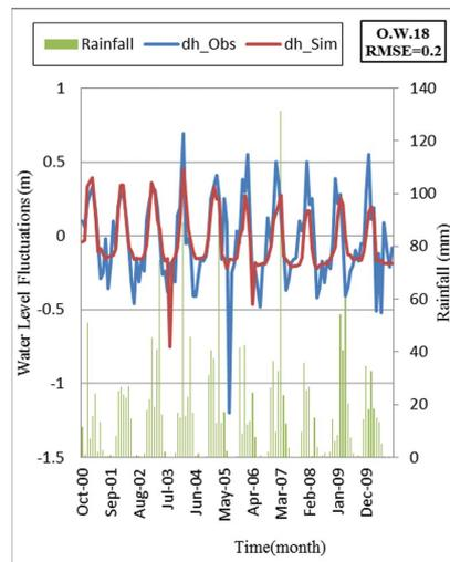
Figure 6. Comparison of observed and simulated water level fluctuation with WTF model for OW18.
