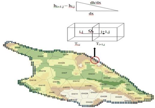
Figure 3. This picture illustrates that how the lateral groundwater inflow or outflow were calculated in boundaries.
