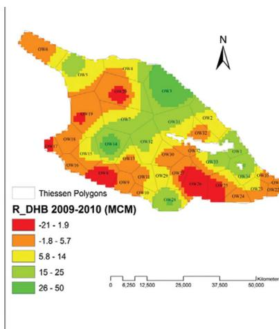
Figure 7. Zoning of Groundwater recharge estimated with DHB method for the year of 2009–2010.
