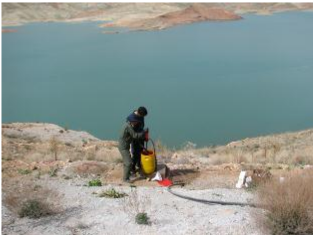
Figure 4. The injection of Rhodamine B into borehole GT 1
