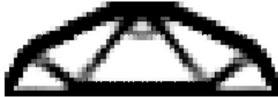
Figure 3 Elimination of undesirable elements in optimal layout of the 2D beam of Figure 2, by employing the noise cleaning method
