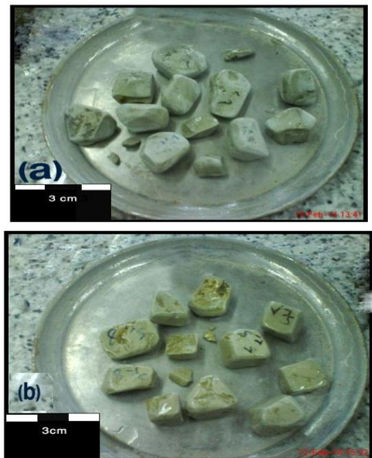
**Fig. 5- Remaining samples after fourth cycle for two types of samples**
