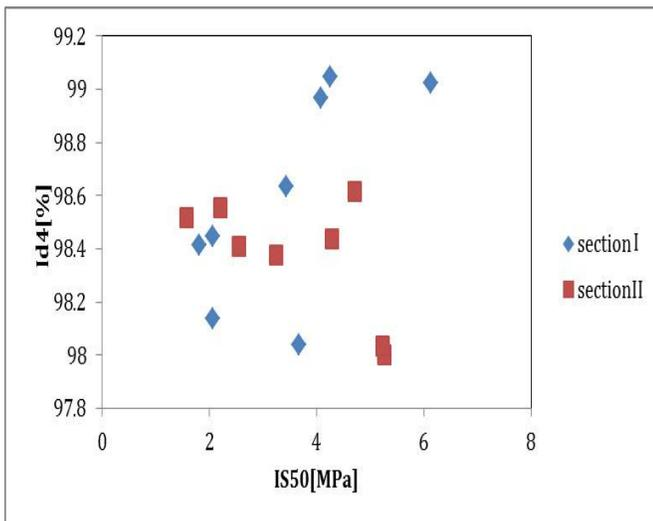
**Fig. 10- Point load index values plotted against slake durability index values after fourth cycle**
