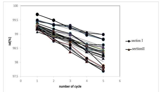
**Fig. 4- Influence of the number of slaking cycles on the slake durability index**
