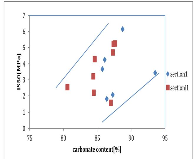
**Fig. 11- Carbonate content plotted against point load index**
