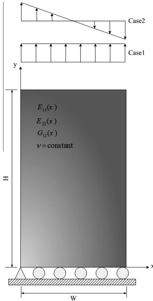
Fig. 6. Rectangular orthotropic FG plate subjected to various loadings.
