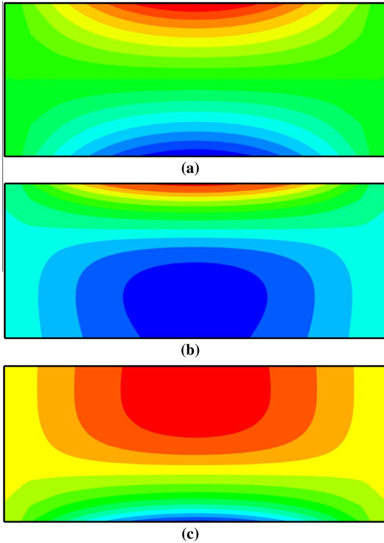
Fig. 21. The axial stress contours for (a)  $E_h/E_0 = 1$  (b)  $E_h/E_0 = 10$  (c)  $E_h/E_0 = 0.1$ .
