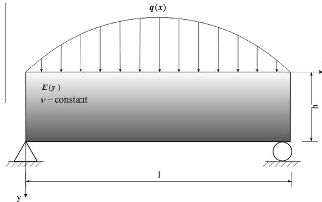
Fig. 17. Geometry and boundary conditions of the FG beam.
