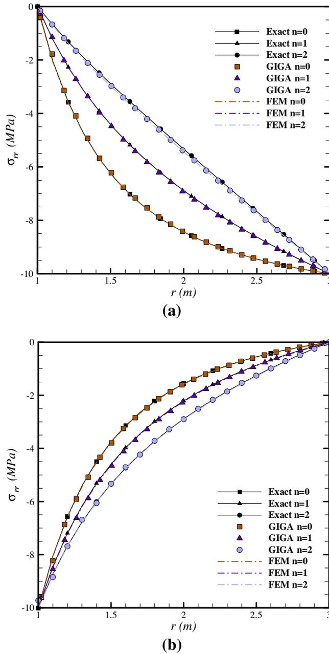
Fig. 12. Radial stress distribution in hollow FG cylinder under (a) internal pressure (b) external pressure.
