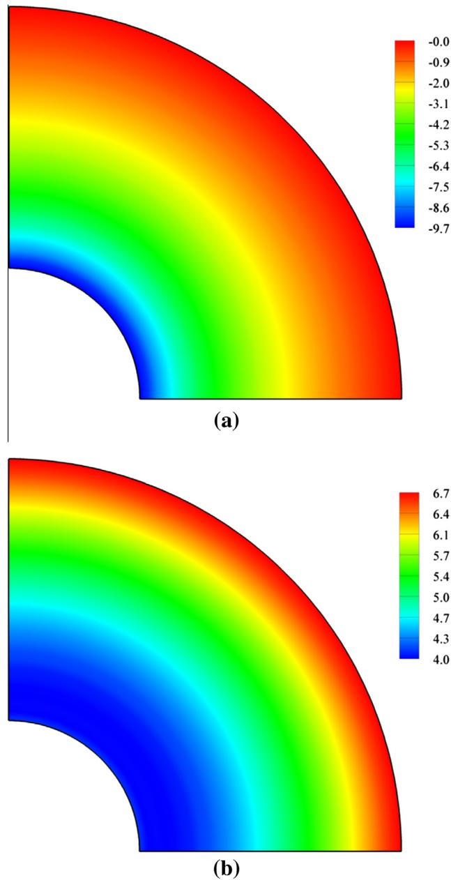
Fig. 14. The contours of the (a) radial, and (b) hoop stress components, for the special case of under internal pressure with  $n = 2$ .
