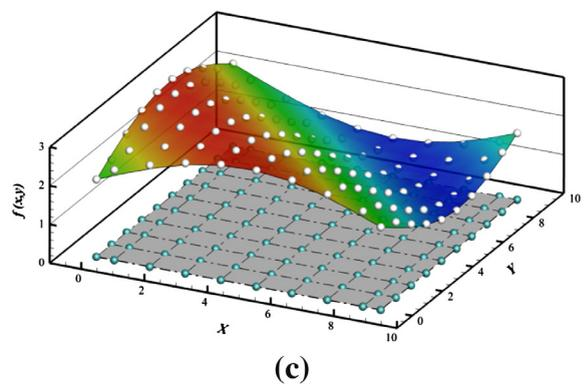
Fig. 3. (a) A typical square domain with the net of control points (b) variations of Young's modulus (c) variations of a typical field variable.
