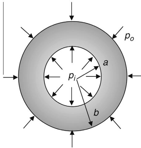
Fig. 10. Hollow cylindrical domain under uniform pressure.
