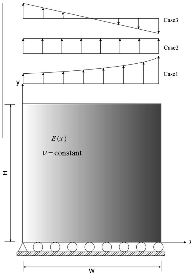
Fig. 4. Square isotropic FG plate subjected to various loadings.
