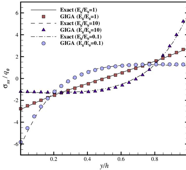
Fig. 19. Distribution of axial stress through the thickness at  $x = l/4$ .
