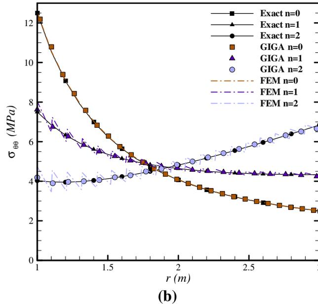
Fig. 13. Hoop stress distribution in hollow FG cylinder under (a) internal pressure (b) external pressure.
