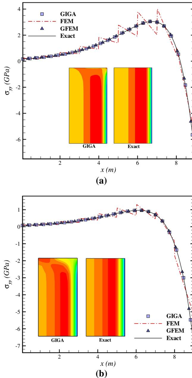
**Fig. 7.** Distribution of  $\sigma_{yy}$  at  $y = 0$  for FG plate subjected to (a) tensile load (b) bending load.
