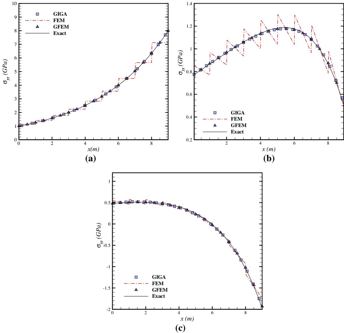
Fig. 5. Distribution of  $\sigma_{yy}$  at  $y = 0$  for FG plate subjected to (a) fixed-grip load (b) tensile load (c) bending load.
