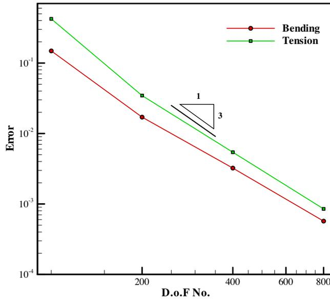
Fig. 8. Errors measured in  $L^2$ -norm of the vertical stress for different loading conditions.
