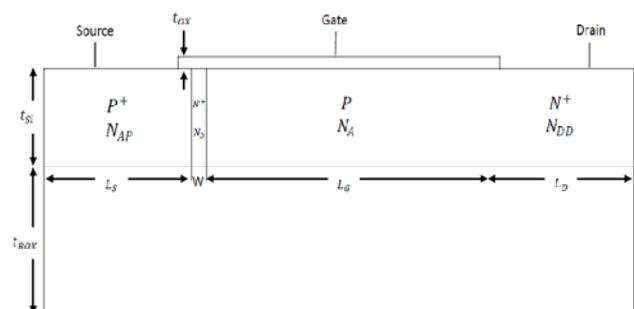
Figure 1. Device structure of the pnin tunnel FET
