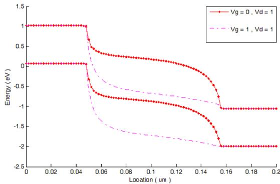
Figure 2. Energy bands for  $W=1$  nm,  $V_{DS}=1$  V,  $V_{GS}=0.1$  V
