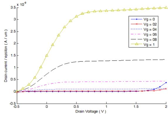
Figure 5. Output characteristics of the tunnel FET for  $W=1$  nm,  $V_{GS}$  is the parameter
