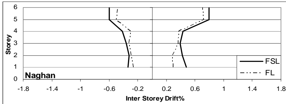
Fig. 10(a) Inter-story drift in the 6-story building
