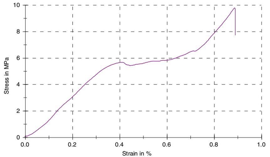
*Mechanical testing.* Four cylindrical specimens of bovine cancellous bone prepared in 2-mm thickness were used for this test. Single-axis pressure test was performed and the specimens were compressed at a strain rate of 0.03 mm/min with a universal machine Zwick Z250 device (Zwick Company, Germany). Results are shown as stress versus strain for strain rate. The compressive modulus of each treatment was taken to be the slope of the stress–strain curve (shown as a schematic diagram in Fig. 2).
