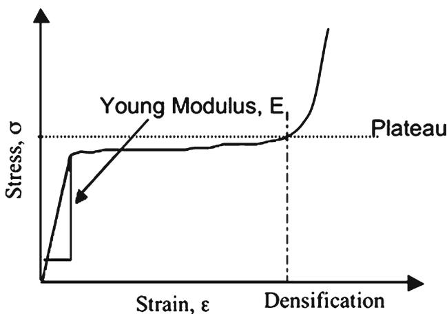
**Figure 2.** Schematic drawing of stress–strain compressive curve.
