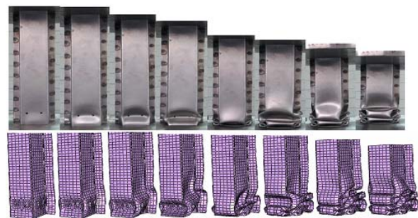
Fig. 15 Comparison of the experimental and numerical results for the specimen with h = 40 and w = 60 mm
