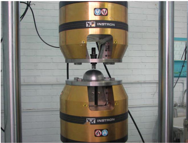
Fig. 13. A serve hydraulic INSTRON 8802 machine in loading on semi-spherical shell by circular bar.
