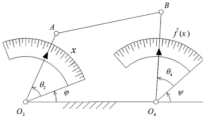
Fig. 2 Indicators of generated function and its variable in terms of the rotation of the follower and crank link
