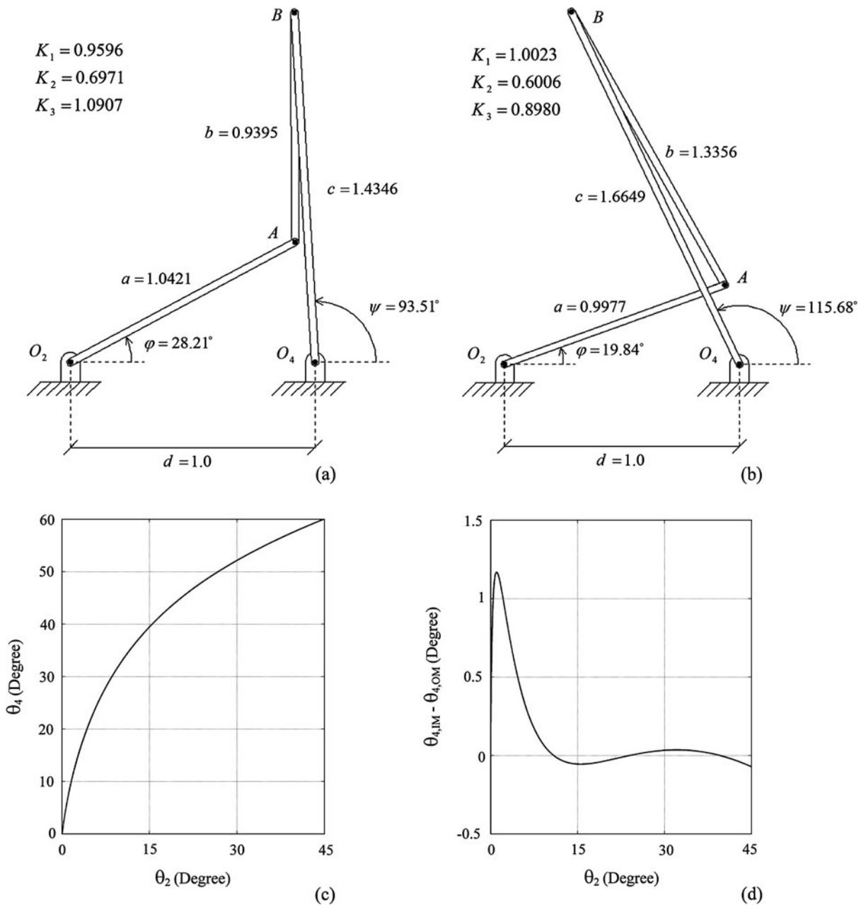
**Fig. 5** Descriptive figures of mechanisms and their related diagrams, (a) initial mechanism, (b) optimum mechanism, (c) desired functions in terms of linkage angle and (d) deviation between follower angle of initial and optimal mechanism
