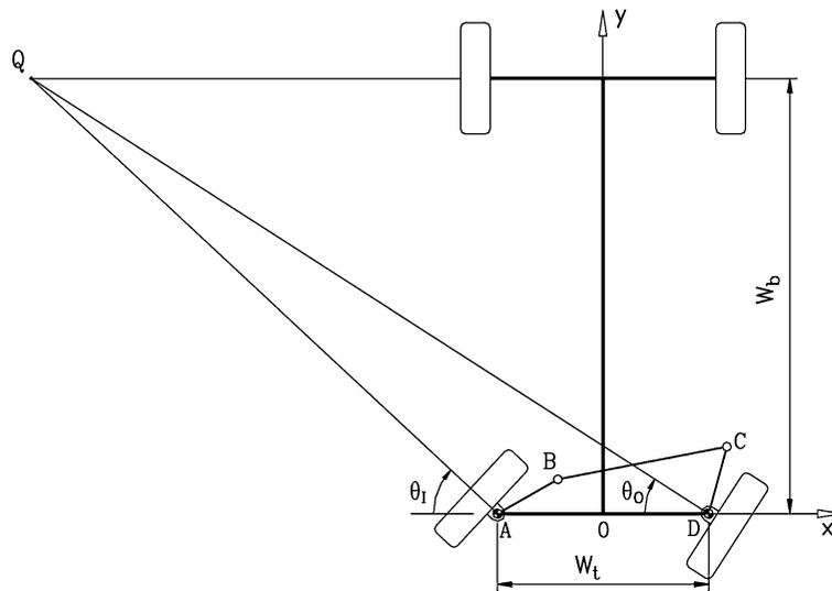
Fig. 3 Ackermann steering linkage [21]
