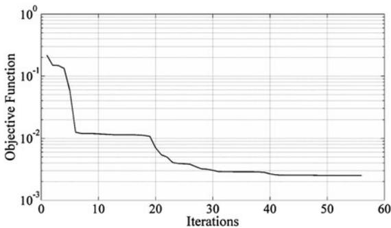
**Fig. 4** History of optimization process for generating logarithm function
