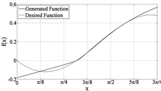
**Fig. 7** Diagrams of generated and desired function with  $f(x) = 0.5(x - 1) \sin x$
