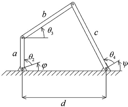
Fig. 1 The schematic plan of the 4R four-bar linkage
