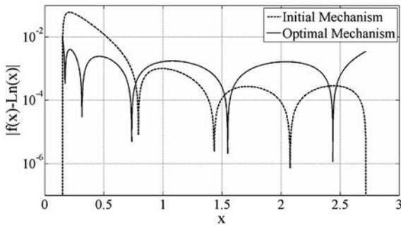
**Fig. 6** Deviation of generated function from logarithm function for initial and optimum mechanism
