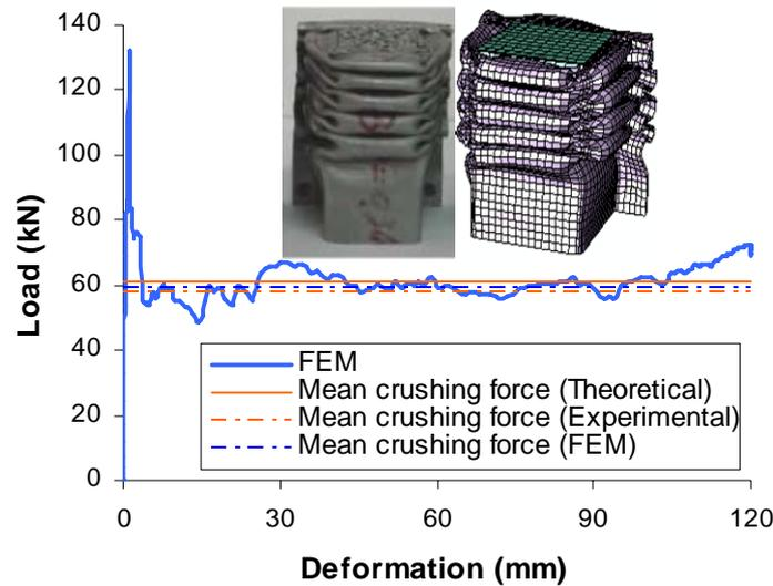
Fig. 3 Comparison of the experimental [5] and numerical result
