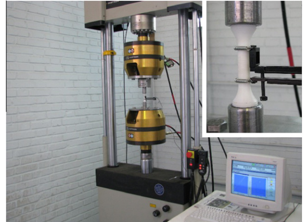
Fig. 3. Servo hydraulic INSTRON 8802 machine.
