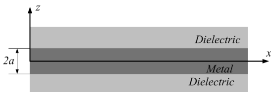
Figure 1. Geometry of a three layer structure, the dielectric layers are assumed to be semi infinite
