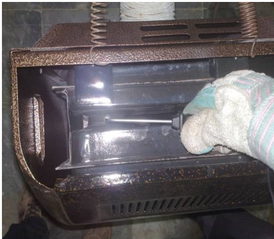
Figure 14. Method of measuring wall temperature
