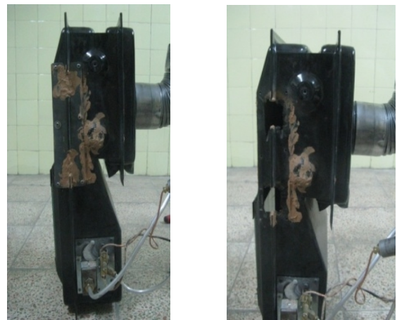
(b)after assembling (a)before assembling Figure 8. The internal body and placement position of inserts
