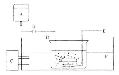
A = Drip, B = Drip control, C = Cooling system, D = Bath, E = Air, F = Water, G = Gut
