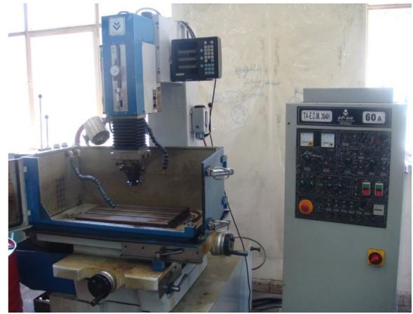
Figure 2: Die-sinking EDM machine used for experiments
