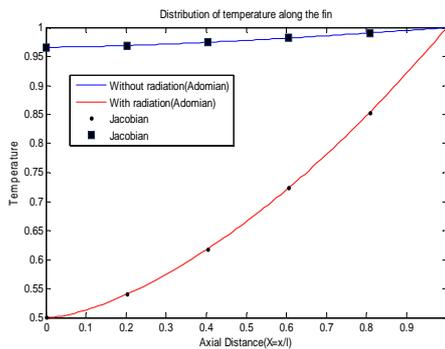
Figure 2. The distribution of axial non-dimensional temperature along the fin ( $\phi=0.8, Ra=202.7, \lambda=12.5, Rd=1.9 \times 10^{-5}, Bi=0.0013, keff=47.6$ )
