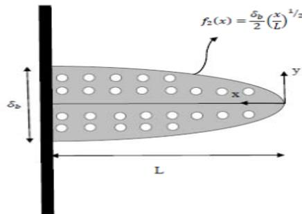
Figure 1. Schematic of a porous fin of convex parabolic close to a vertical constant temperature wall.
