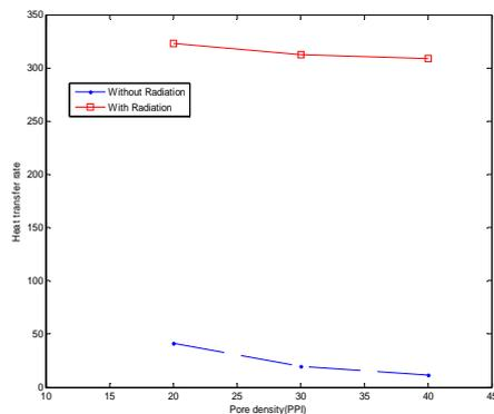
Figure 4. The effects of PPI on heat transfer rate with and without radiation effect.
