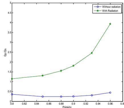
Figure 5. The plot of heat transfer ratio of porous fin to solid fin vs. porosity
