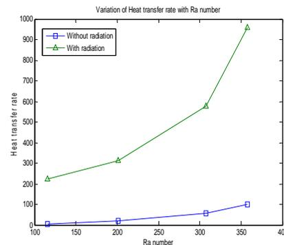
Figure 3. The variation of heat transfer rate with Ra number with and without radiation effect.
