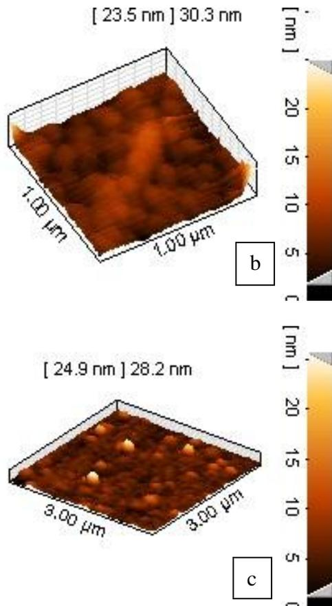
Fig.4. 3D- view of AFM topography of DSPC with and without cholesterol at different concentration of lipid/cholesterol (a)S1, (b)S2, (c)S3
