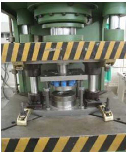
Fig. 3 Hydraulic press and die set used for experiments
