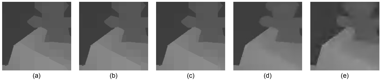
Figure 3. A part of compressed depth image of Teddy with \text{bpp} \approx 0.15 which compressed with (a) constant and wedge functions (b) constant, wedge and linear functions (c) constant, wedge, linear and plate functions (d) H264 (e) JPEG2000
