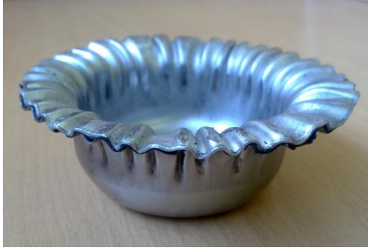
Fig. 3 Sample of laminated sheet after forming
