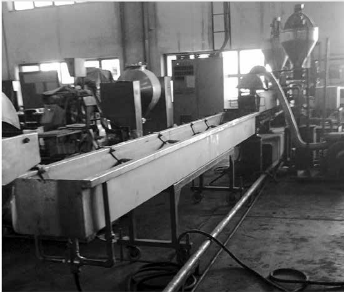
Figure 2. The twin screw extruder for applying shearing action during devulcanization
