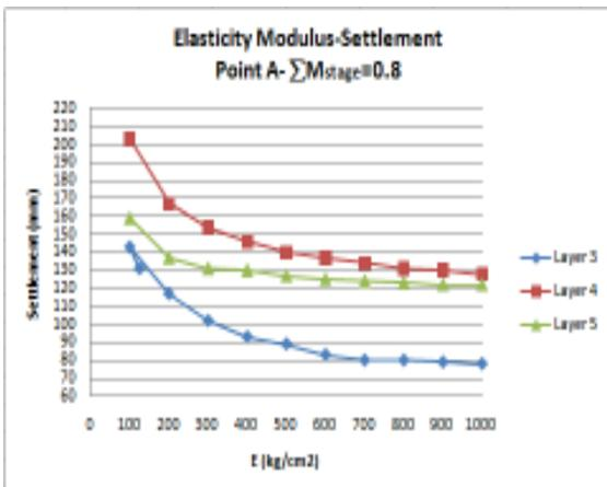
Figure 5: Changes in the subsidence of A point
