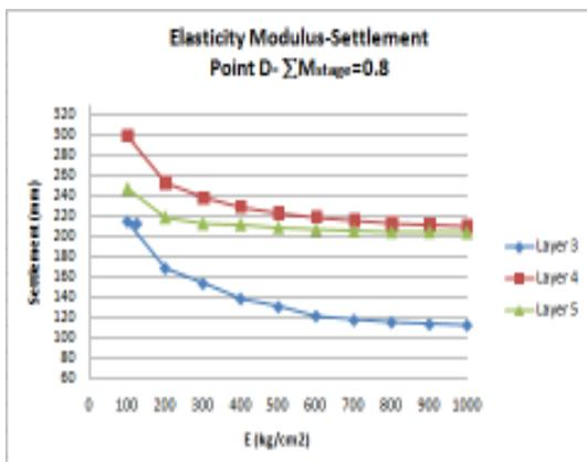
Figure 6: Changes in the subsidence of D point
