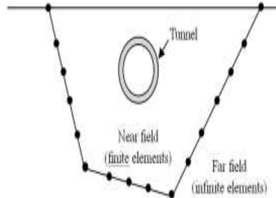
**Figure 1: Schematic of the finite/infinite element approach**
