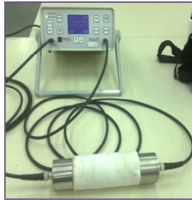
Figure 5. A view of V_{pl} measurement on intact rock sample with the PUNDIT ultrasonic apparatus.
