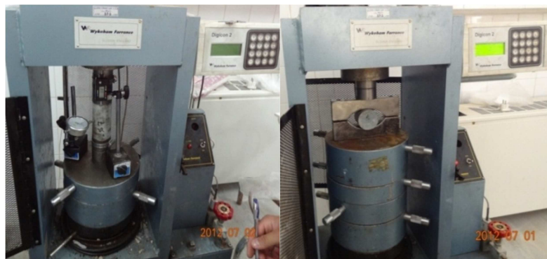
Figure 4. Device of left) uniaxial compressive strength test and right) Brazilian test
