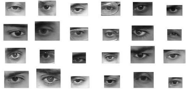
Figure 6. Open-eye template examples with various sizes of the eye, luminance changes, with or without glasses
