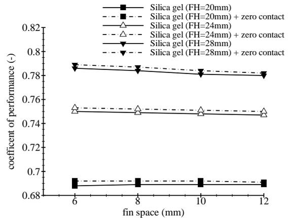
Fig 9: The variation of coefficient of performance with fin space for different fin heights for the bed with and without thermal contact resistance
