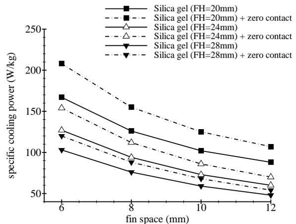
Fig 10: The variation of specific cooling power with fin space for different fin heights for the bed with and without thermal contact resistance
