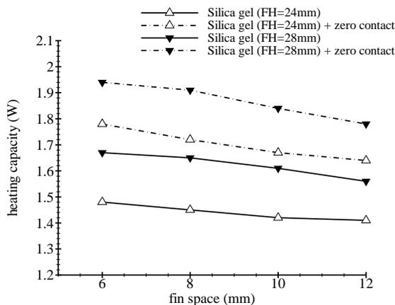
Fig 7: The variation of heating capacity with fin for different fin heights in the bed with and without thermal contact resistance
