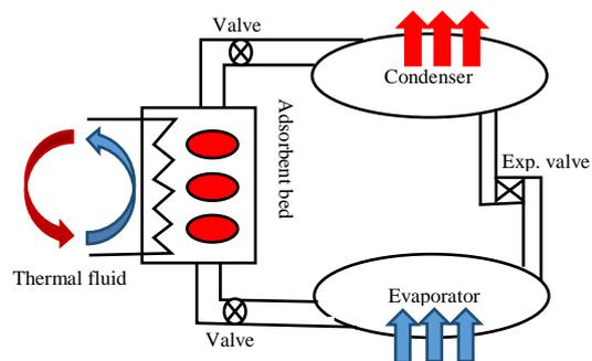
Fig 1: Schematic of an adsorption system
