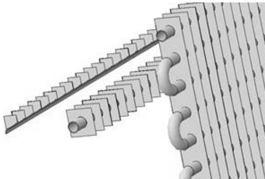
Fig 2: Schematic of adsorbent bed with numerical modeling domain
