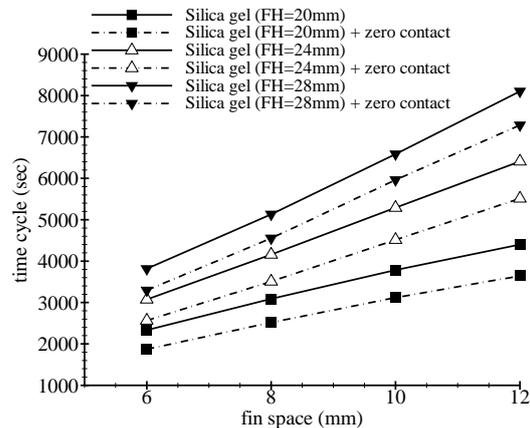
Fig 6: The variation of cycle time with fin space for different fin heights in the bed with and without thermal contact resistance
