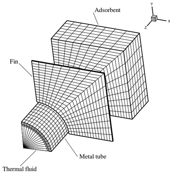
Fig 4: Schematic of the grid system
