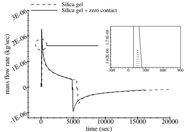
Fig 5: Time variation of total mass flow for beds with and without thermal contact resistance
