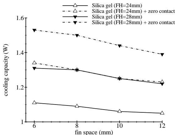
Fig 8: The variation of cooling capacity with fin space for different fin heights in the bed with and without thermal contact resistance
