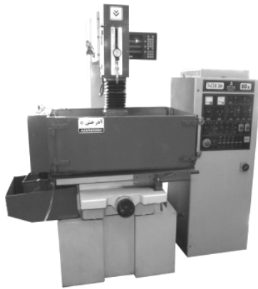
Figure (1) Die-sinking EDM machine used for experiments
