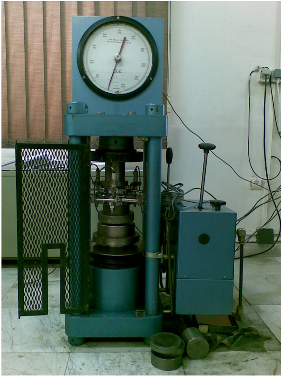
Fig. 2. Uniaxial compressive test machine for determination of UCS and E_s .
