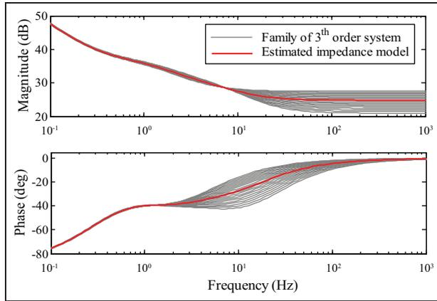
**Figure 4.** Impedance Bode plot of a family of third-order system and estimated model.
