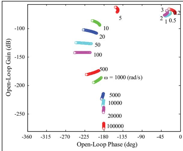
Figure 8. The boundary of the plant templates.
