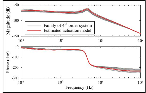
**Figure 6.** Bode plot of a family of the fourth-order actuation system and the estimated model.
