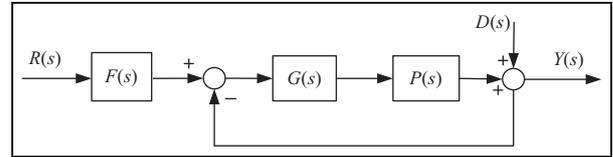
**Figure 7.** A two-degree-of-freedom feedback system.
