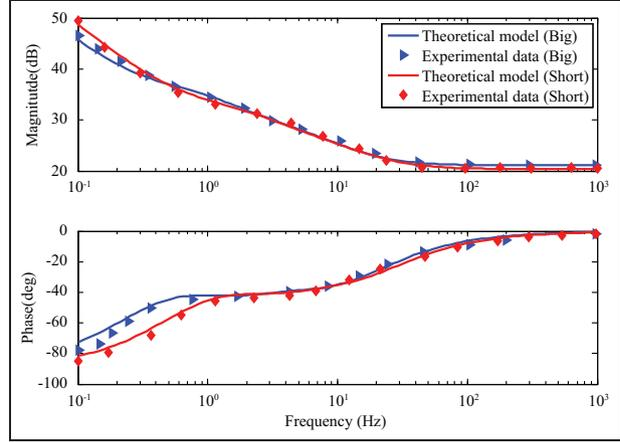
**Figure 3.** Comparison of the experimental impedance responses with the theoretical model.
