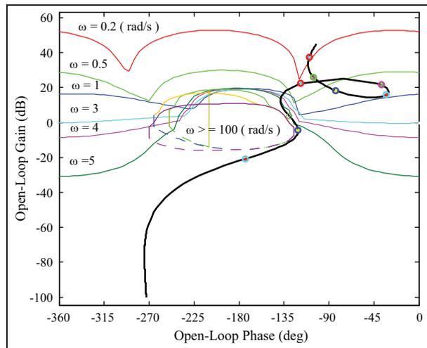
Figure 9. QFT bounds and loop shaping of  $L(s)$  on the NC. QFT: quantitative feedback theory; NC: Nichols chart.
