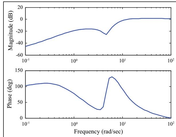
**Figure 14.** Bode plot of sensitivity function,  $S(j\omega)$ .
