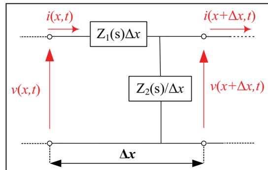
**Figure 2.** Equivalent single-unit circuit.
