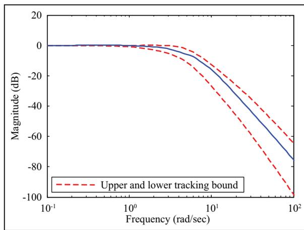
**Figure 13.** The closed-loop frequency response of the uncertain plant with the upper and lower tracking bounds with pre-filter.
