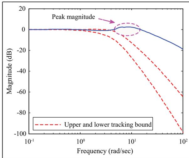
**Figure 12.** The closed-loop frequency response of the uncertain plant with the upper and lower tracking bounds without pre-filter.
