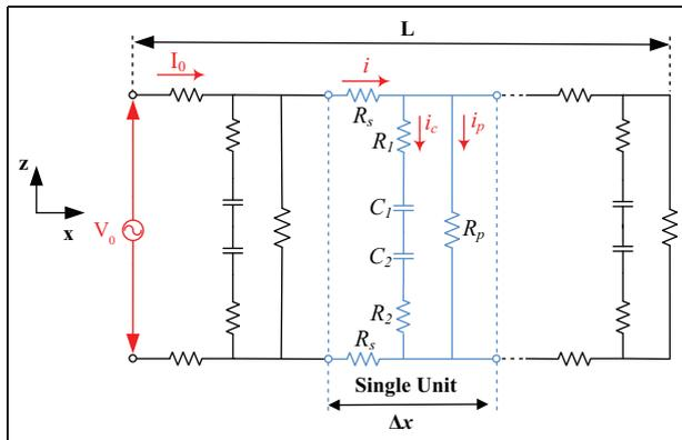
**Figure 1.** Distributed RC model of an IPMC actuator. RC: resistance–capacitance; IPMC: ionic polymer metal composite.
