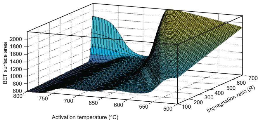
**Figure 8.**  $S_{\text{BET}}$  versus activation temperature and  $\text{ZnCl}_2$  agent ratio at an activation time of 60 minutes and heating rate of  $5^\circ\text{C}/\text{minute}$ .
