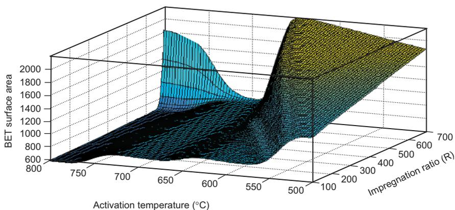
**Figure 9.**  $S_{\text{BET}}$  versus activation temperature and  $\text{ZnCl}_2$  agent ratio at an activation time of 60 minutes and heating rate of  $30^\circ\text{C}/\text{minute}$ .
