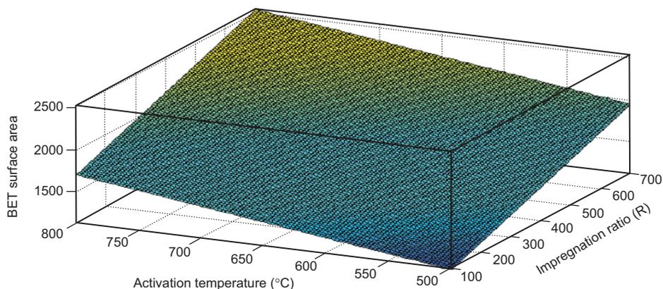
**Figure 7.**  $S_{\text{BET}}$  versus activation temperature and KOH impregnation ratio at an activation time of 60 minutes and heating rate of 30 °C/minute.
