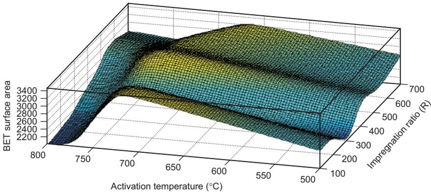
Figure 6.  $S_{BET}$  versus activation temperature and KOH impregnation ratio at an activation time of 60 minutes and heating rate of  $5^{\circ}C/minute$ .
