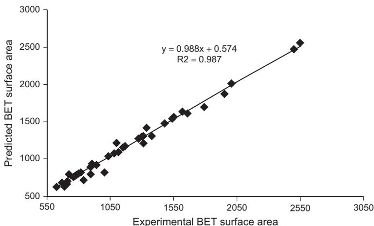
**Figure 11.** Comparison of the predicted and real  $S_{\text{BET}}$  data for ACs produced from a cellulose-based precursor.
