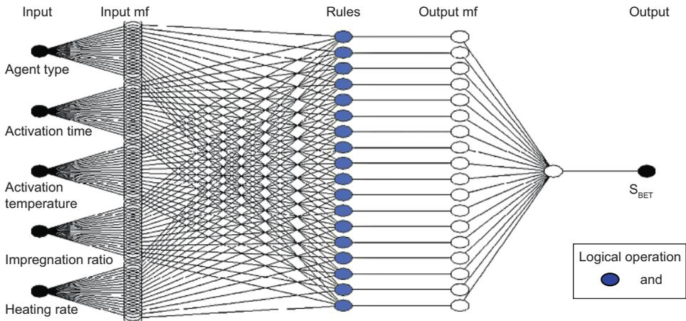
**Figure 3.** Structure of the proposed ANFIS model for predicting BET surface area of ACs.
