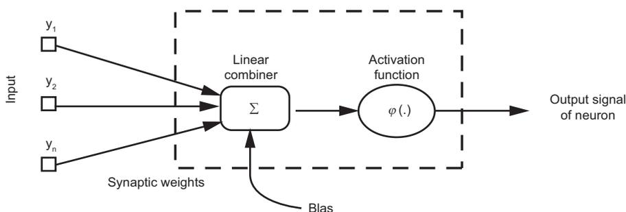
**Figure 2.** Schematic representation of a projection-based neuron.
