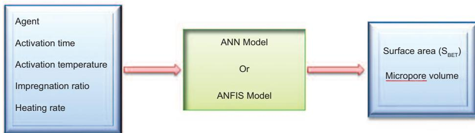
**Figure 1.** Block diagram of the calculation procedure.
