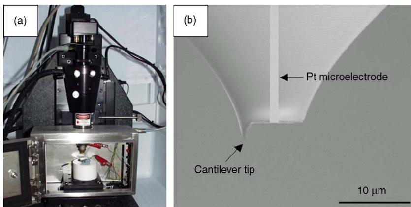
Fig. 1. (a) The AFM instrument and electrochemical cell. (b) The dual mode probe for integrated EC-AFM/SECM measurement.
