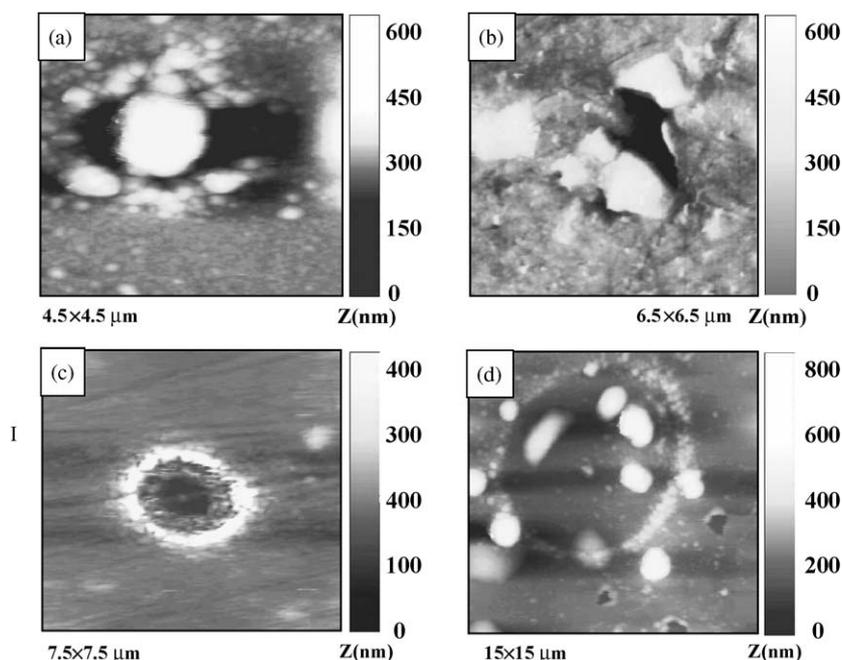
Fig. 2. EC-AFM topography of an Al–Si alloy under anodic polarisation close to breakdown potential in 10 mM NaCl + 50 mM KI solution; (a)–(d) different surface areas.
