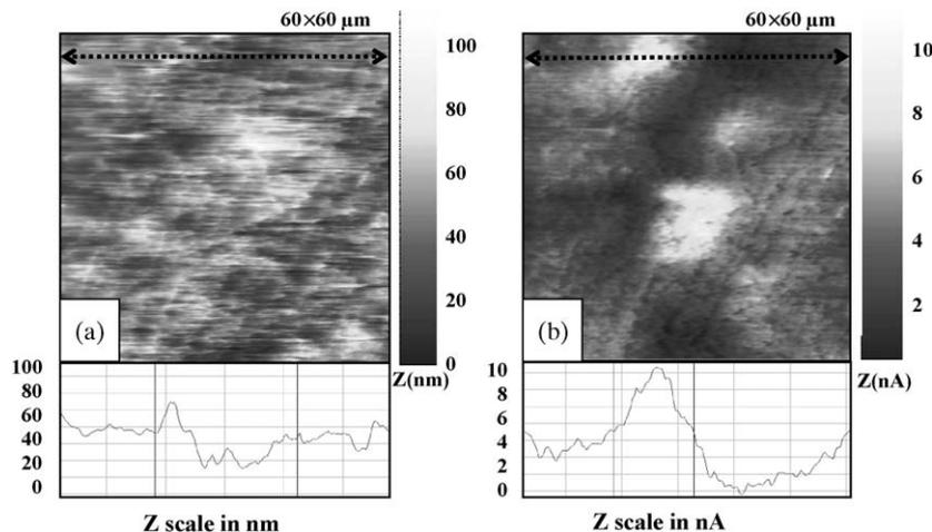
Fig. 4. Concurrent EC-AFM/SECM images obtained for pure aluminium in 10 mM NaCl + 5 mM KI at 50 mV anodic polarization. (a) AFM topography and line profile. (b) SECM electrochemical current map and line profile.
