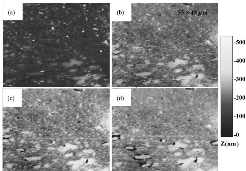
Fig. 3. In situ AFM topography of an Al–Mn–Cu–Cr–Zr alloy with an Al–Si braze cladding layer (after heat treatment at 600 °C) during free immersion in 10 mM NaCl + 50 mM KI solution for 6 h. Sequence from (a) to (d) show trench formation.
