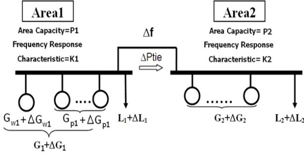
**Fig. 1** schematic diagram of the test system.
