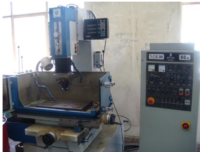
Fig. 2 Die-sinking EDM machine used for experiments
