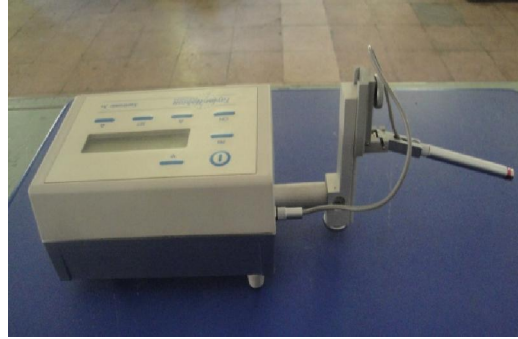
Fig. 3 Digital surface roughness tester and electronic balance
