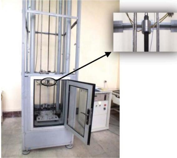
Figure 9. Drop-weight test device and the accelerometer.
